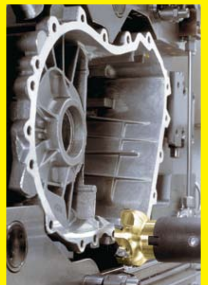
CoroMill Century is an innovative, lightweight face mill cutter for fast, precision machining of aluminium gearbox housings.
