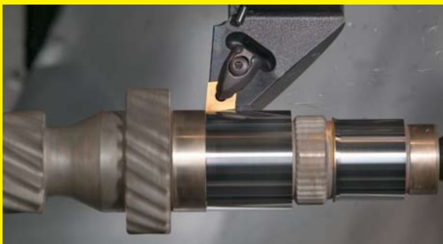
Optimized wiper inserts in CB7015 with Safe-Lok multi-corner technology make a strong choice for balancing surface and dimensional tolerance with productivity demands.
