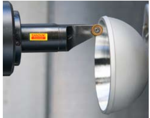
Holder: A20M-SRXDL 08-R Insert: R300-0828E-PL 1030
