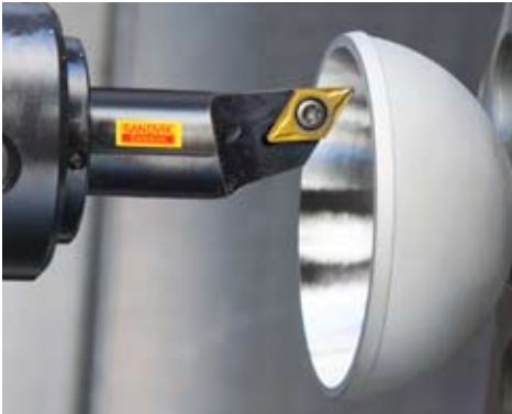
Holder: A20M-ADXCL 11-R Insert: DCGT 11T308-UM 1025
